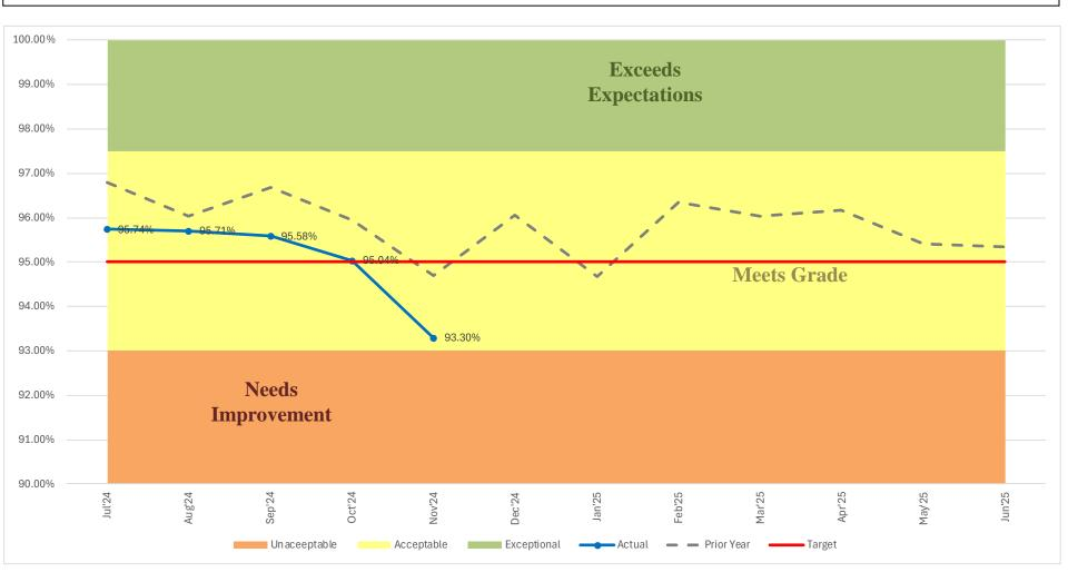
Rail Mean Distance Between Failures measured as the average rail car miles between NTD reportable mechanical failures, i.e., those precluding a rail car from completing its revenue trip or starting its next scheduled revenue trip.
